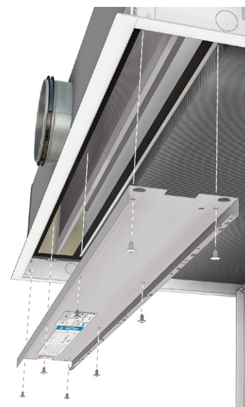
Picture 5. Cleaning hatch off.
